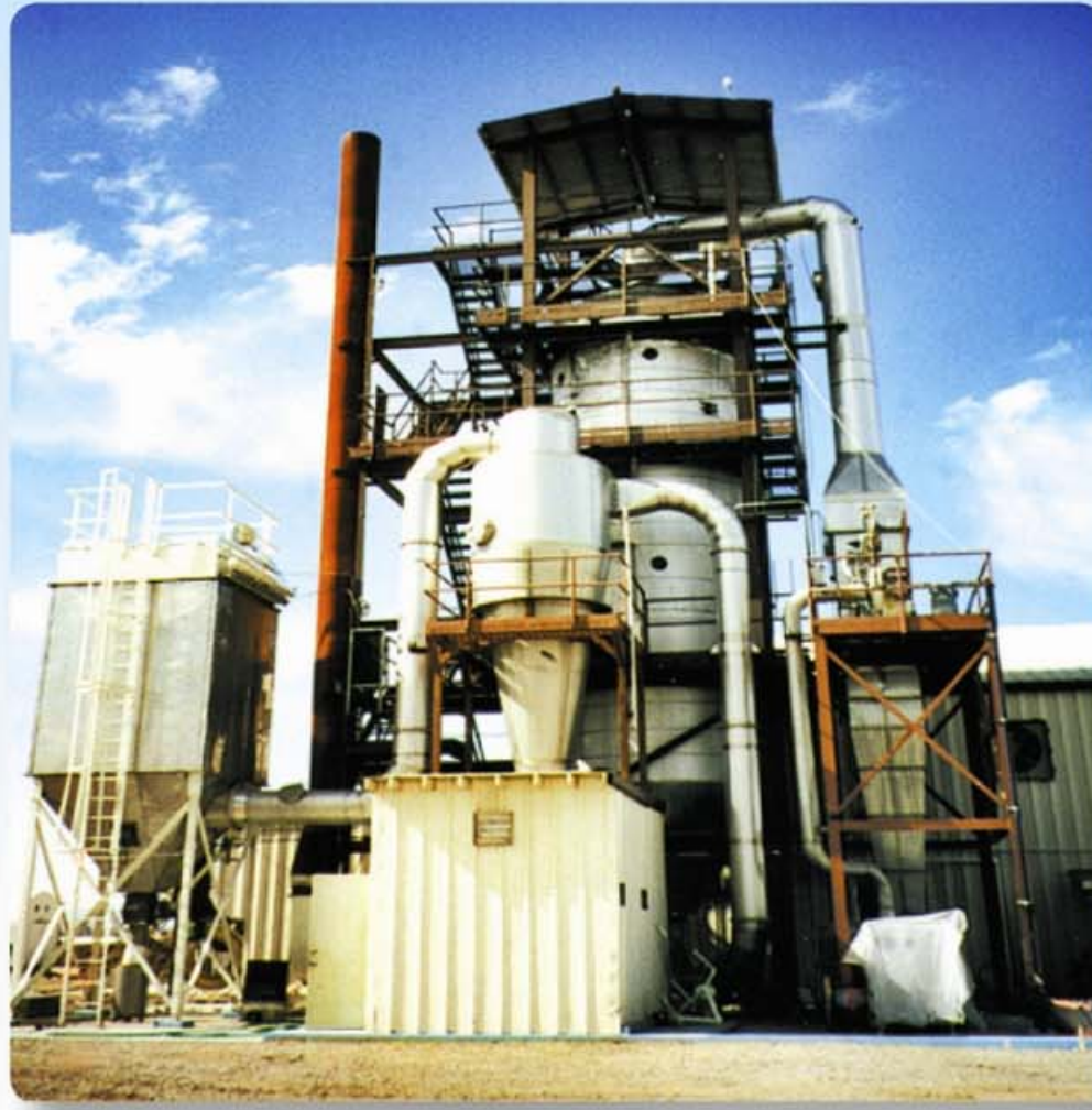
Harvested Spirulina Is Dried Within Couple Of Seconds In This 4-storey High Drying Chamber, Preserving Its Full Potency.
